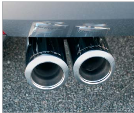
Sport rear silencer with twin tail pipe i 35 08 005, round, chrome-finished.
