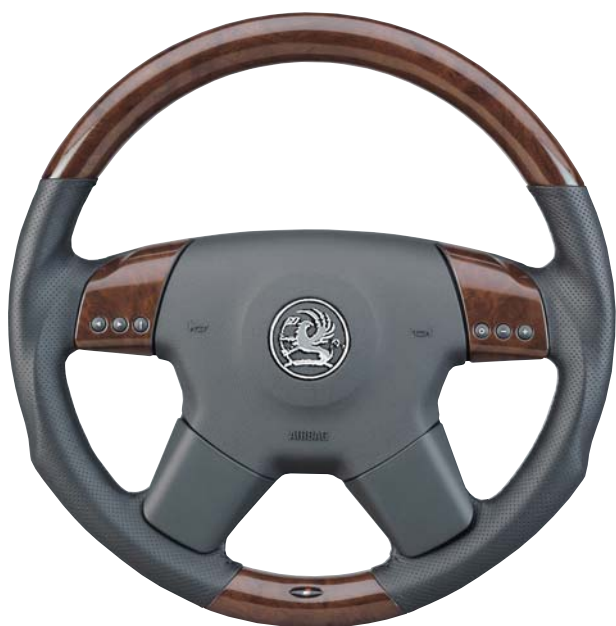
Steering wheel in river elm wood-effect/leather i 71 18 149 with spoke cover trims in river elm wood-effect i 34 17 040.
