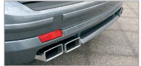
Vectra Estate: Bumper protection strips i 34 01 030, dual branched twin-rear silencer i 34 08 044/132 with rear lower skirt i 34 01 464. (Not pictured: rear silencer i 34 08 054/046/047 with twin tailpipes and rear lower skirt i 34 01 463; rear lower skirt i 34 01 473/474 with OE parking distance sensor.)
