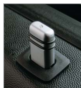
Chrome rings i 32 17 020 for heating/ventilation switches.
