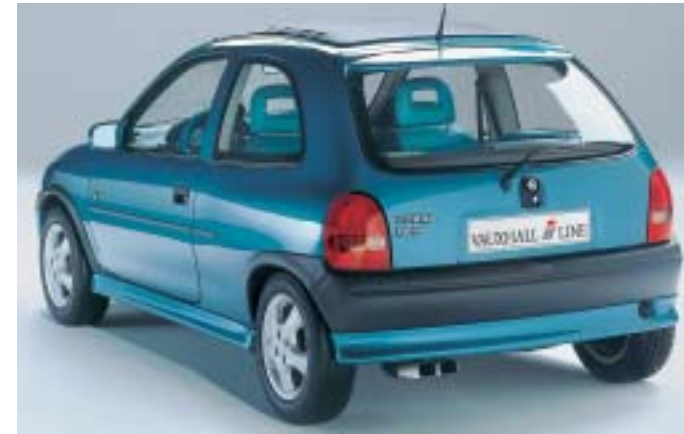
Roof spoiler i 12 01 448, rear skirt i 12 01 451 (up to M.y. '97,5), side sill set i 12 01 302, rear silencer i 12 08 001.
